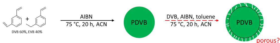
Figure 33: Schematic depiction of precipitation polymerization of DVB in acetonitrile followed by the attempt to PDVB porous shell growth by addition of a porogen in the second reaction step as suggested by literature (here: toluene). 85
