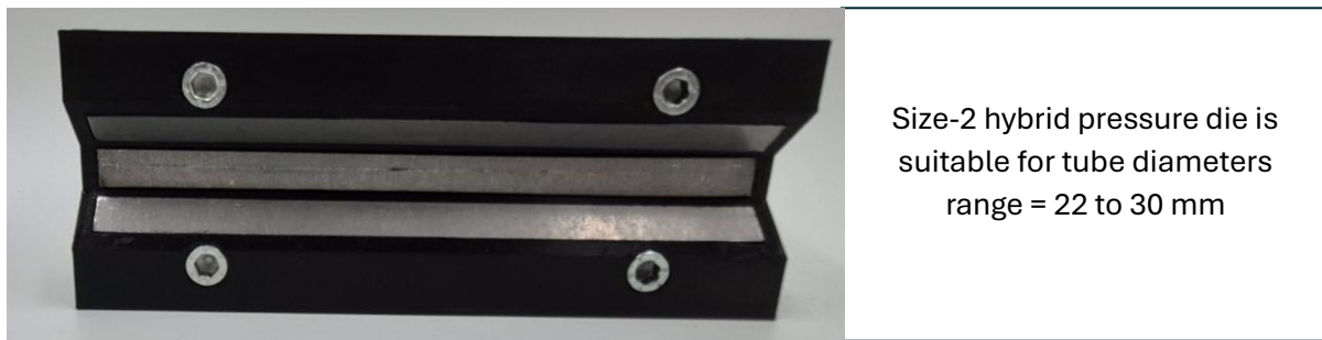
Figure 10.1 : Standardization of hybrid tools according to the aspect ratio and size factor ( S_f )
