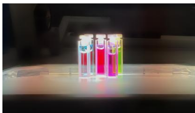
Figure 4.13. Experimental setup for photostability measurements. The sample solutions were placed vertically in quartz cuvettes on top of the overhead projector.
